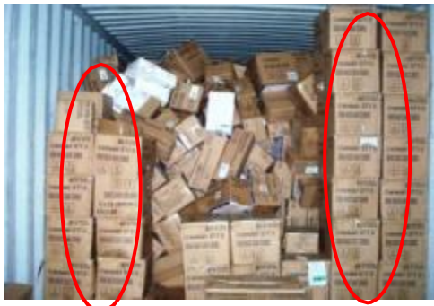
Figure 3: INCORRECT METHOD - Cartons were column stacked and not secured. Load shifted in transit.
